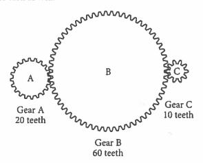
If Gear A is rotated by the motor at a rate of 100 rpm, what is the number of revolutions per minute for Gear C?
